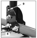
NOTE: Orientation of handle assemblies to frame will depend on how the operator wishes to operate snap button (9). If snap button is assembled to outside of the generator frame the fingers will operate it. If snap button is assembled to inside of the generator frame the thumbs will operate it. The figure shows the snap button assembled to inside of generator frame
